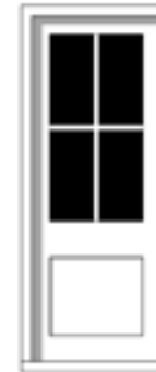
4 lite pane glazing over single panel
